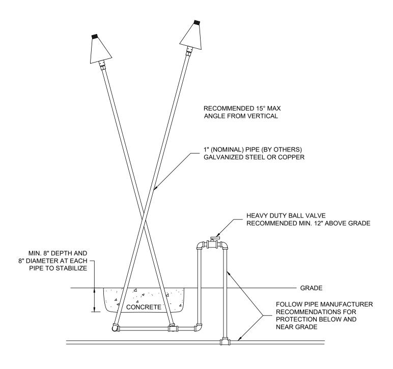
INSTALLATION STYLE SHOWN IS ONLY AN EXAMPLE. CONSULT A LICENSED PLUMBER AND FOLLOW APPLICABLE CODES FOR GAS PIPE LAYOUT AND INSTALLATION.
