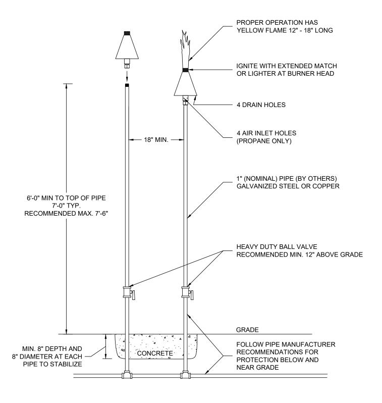
INSTALLATION STYLE SHOWN IS ONLY AN EXAMPLE. CONSULT A LICENSED PLUMBER AND FOLLOW APPLICABLE CODES FOR GAS PIPE LAYOUT AND INSTALLATION.
